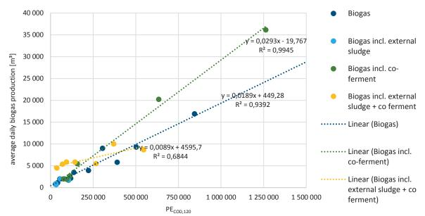
Figure 28 - Average daily biogas production [m3] vs. PEcod,120, n=27
