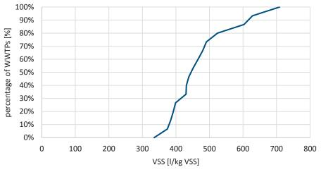
Figure 27 – Specific biogas production in relation to fed VSS [I/kg VSS], n=16
