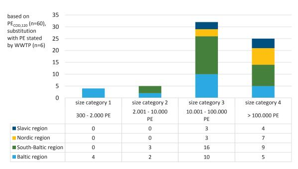
Figure 2 – WWTPs grouped by size according to HELCOM recommendation 28E/5 (2007) and region
