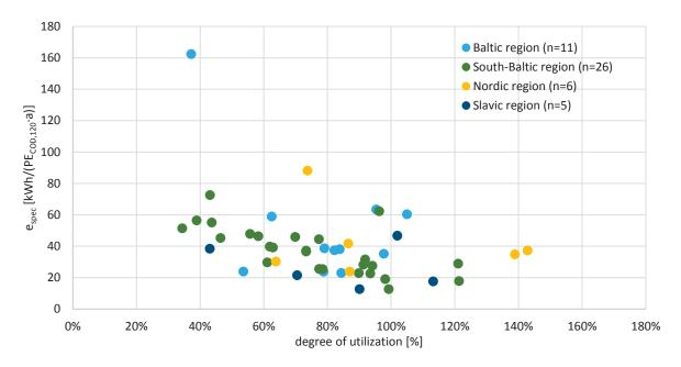
Figure 21 – Specific energy consumption [kWh/(PEcoD,120·a)] in relation to degree of utilization
