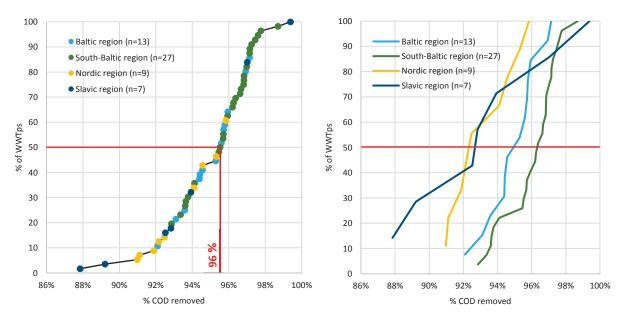
Figure 12 - Overall COD removal efficiency
