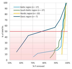
Figure 16 - Overall P removal efficiency
