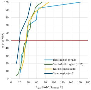
Figure 18 – Specific energy consumption [kWh/( $PE_{COD,120}$ ·a)], accumulative
