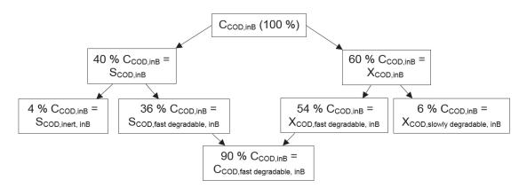
Figure 31 – Fractionation of the chemical oxygen demand according to Sieker [2018]
