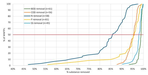
Figure 11 - Nutrient removal efficiency
