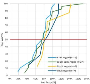
Figure 8 – Degree of utilization based on COD, accumulative
