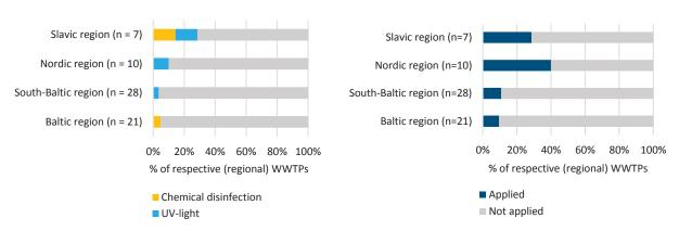
Figure 6 – Applied disinfection methods
