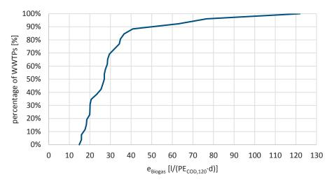
Figure 26 – Specific biogas production [I/(PEcod,120·d)], n=27
