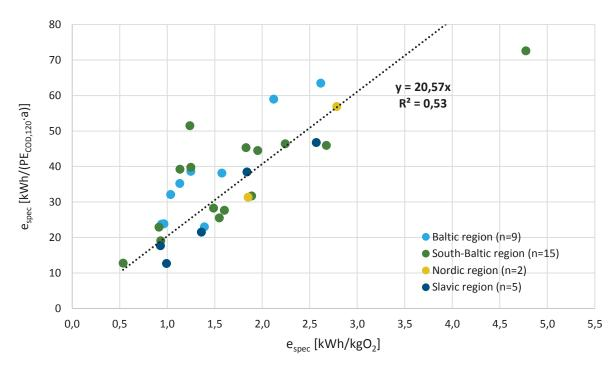
Figure 25 - Specific energy consumption kWh/kgO₂ in relation to kWh/(PE<sub>COD,120</sub>·a)
