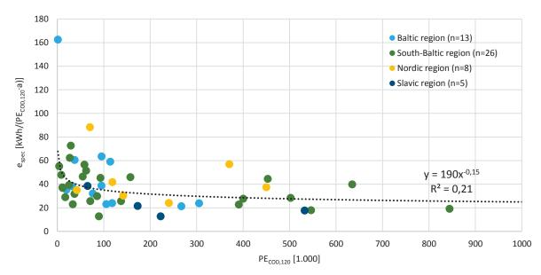
Figure 20 – Specific energy consumption [kWh/(PE<sub>COD,120</sub>·a)] in relation to connected PE [PE<sub>COD,120</sub>]
