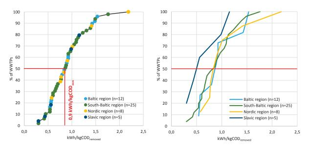
Figure 22 – Specific energy consumption [kWh/kgCODrem], accumulative
