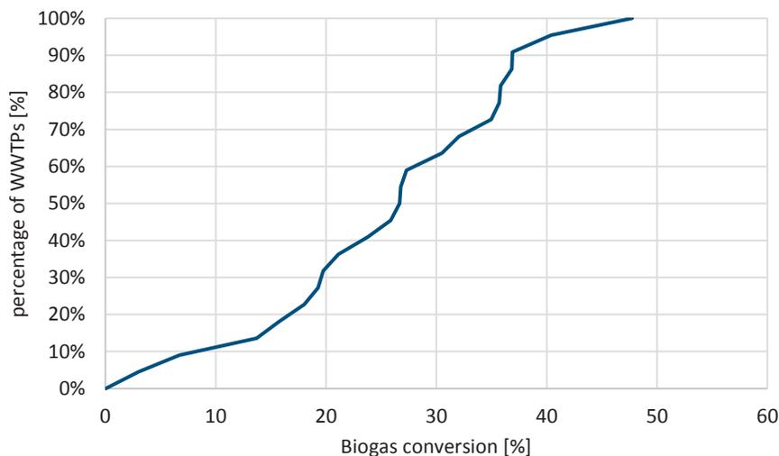
Figure 29 – Rate of biogas conversion into electrical energy, n=23
