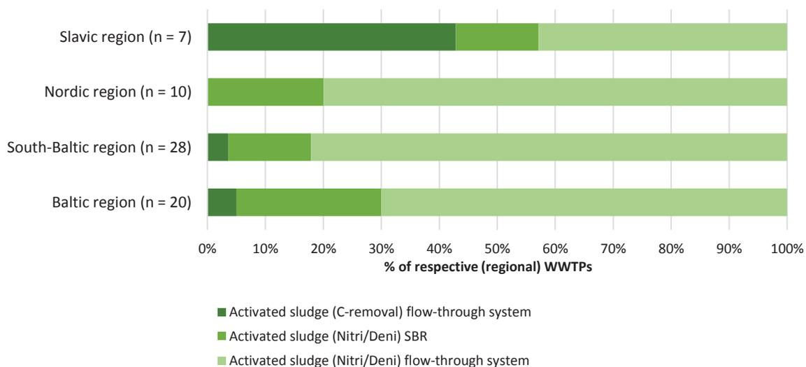
Figure 3 – Applied wastewater treatment technologies
