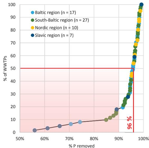
Figure 16 – Overall P removal efficiency
