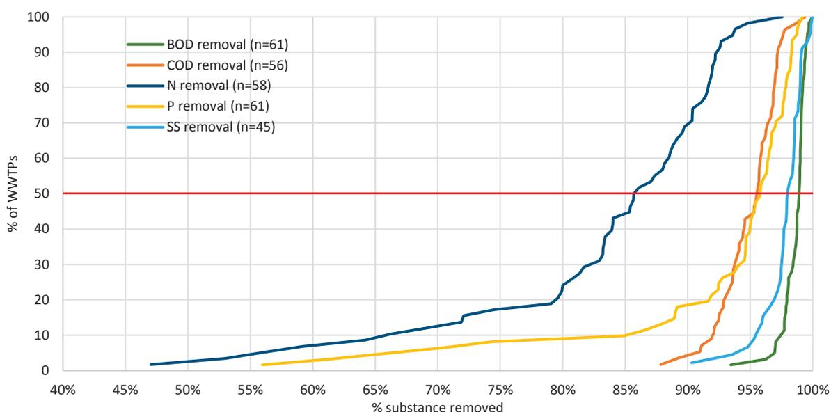
Figure 11 – Nutrient removal efficiency
