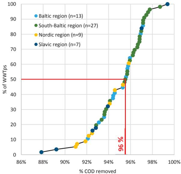
Figure 12 – Overall COD removal efficiency
