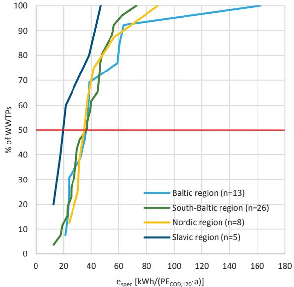
Figure 19 – Specific energy consumption [kWh/(PE<sub>COD,120</sub>·a)], regionalised
