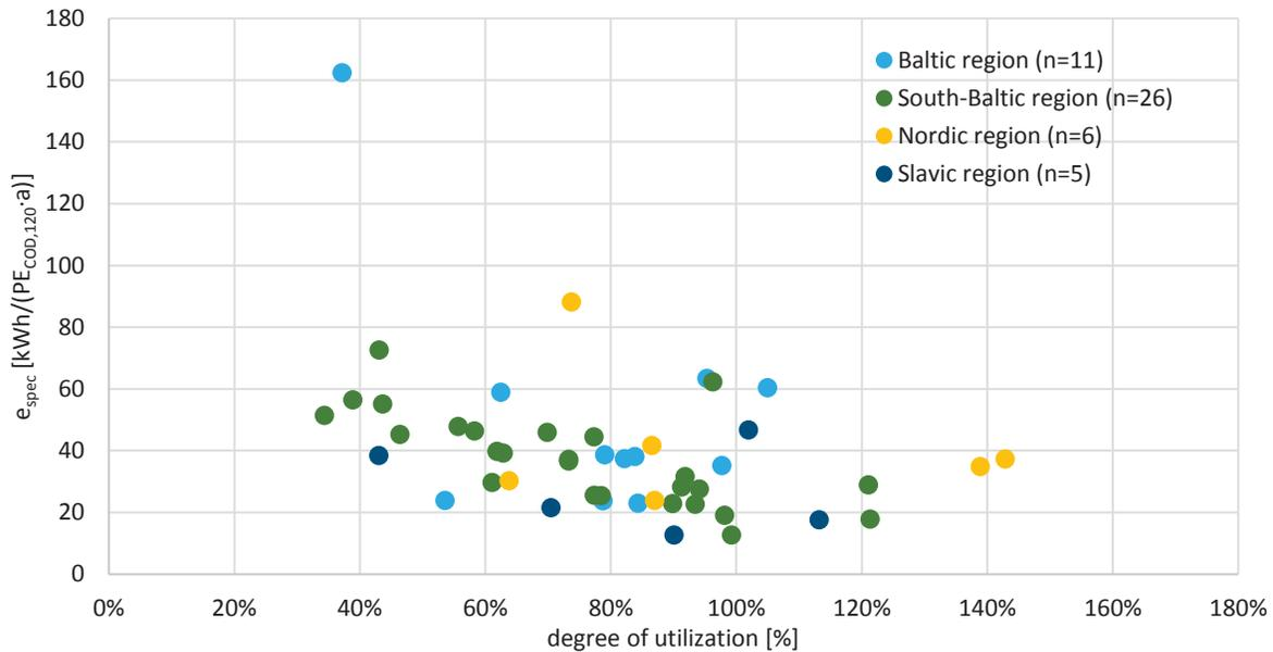
Figure 21 – Specific energy consumption [kWh/(PE<sub>COD,120 a</sub>)] in relation to degree of utilization
