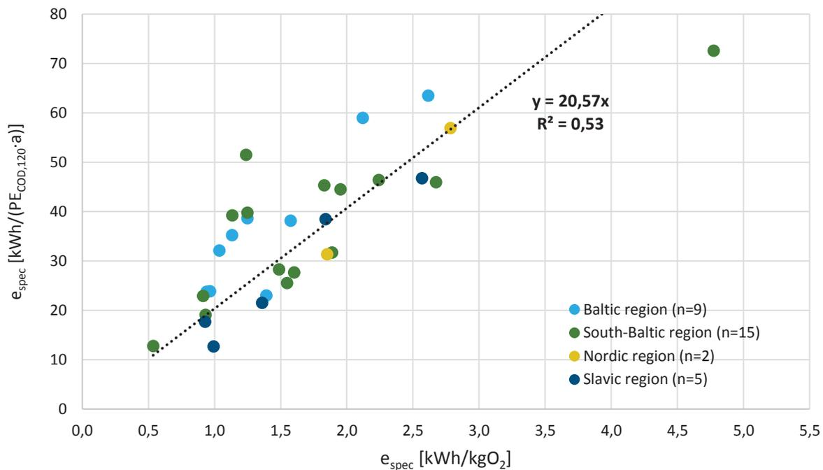
Figure 25 – Specific energy consumption kWh/kgO<sub>2</sub> in relation to kWh/(PE<sub>COD,120·a</sub>)
