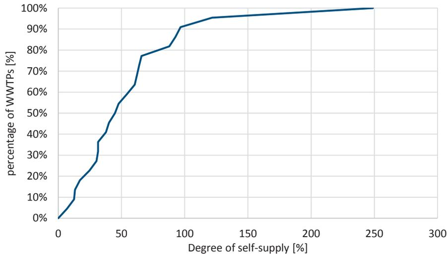
*Figure 30 – Degree of self-supply of electrical energy, n=23*
