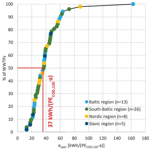
Figure 18 – Specific energy consumption [kWh/(PE<sub>COD,120</sub>·a)], accumulative
