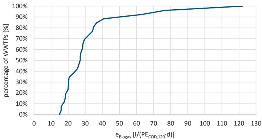
Figure 26 – Specific biogas production [l/(PE<sub>COD,120</sub>·d)], n=27
