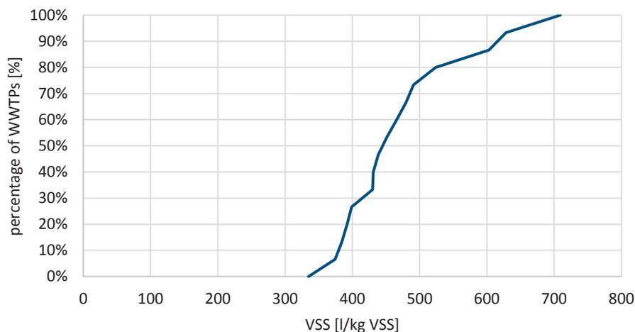
Figure 27 – Specific biogas production in relation to fed VSS [l/kg VSS], n=16
