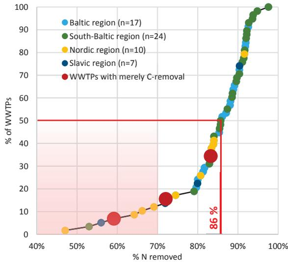
Figure 14 – Overall N removal efficiency
