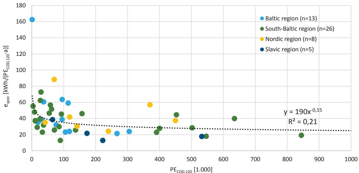
Figure 20 – Specific energy consumption [kWh/(PE<sub>COD,120</sub>·a)] in relation to connected PE [PE<sub>COD,120</sub>]
