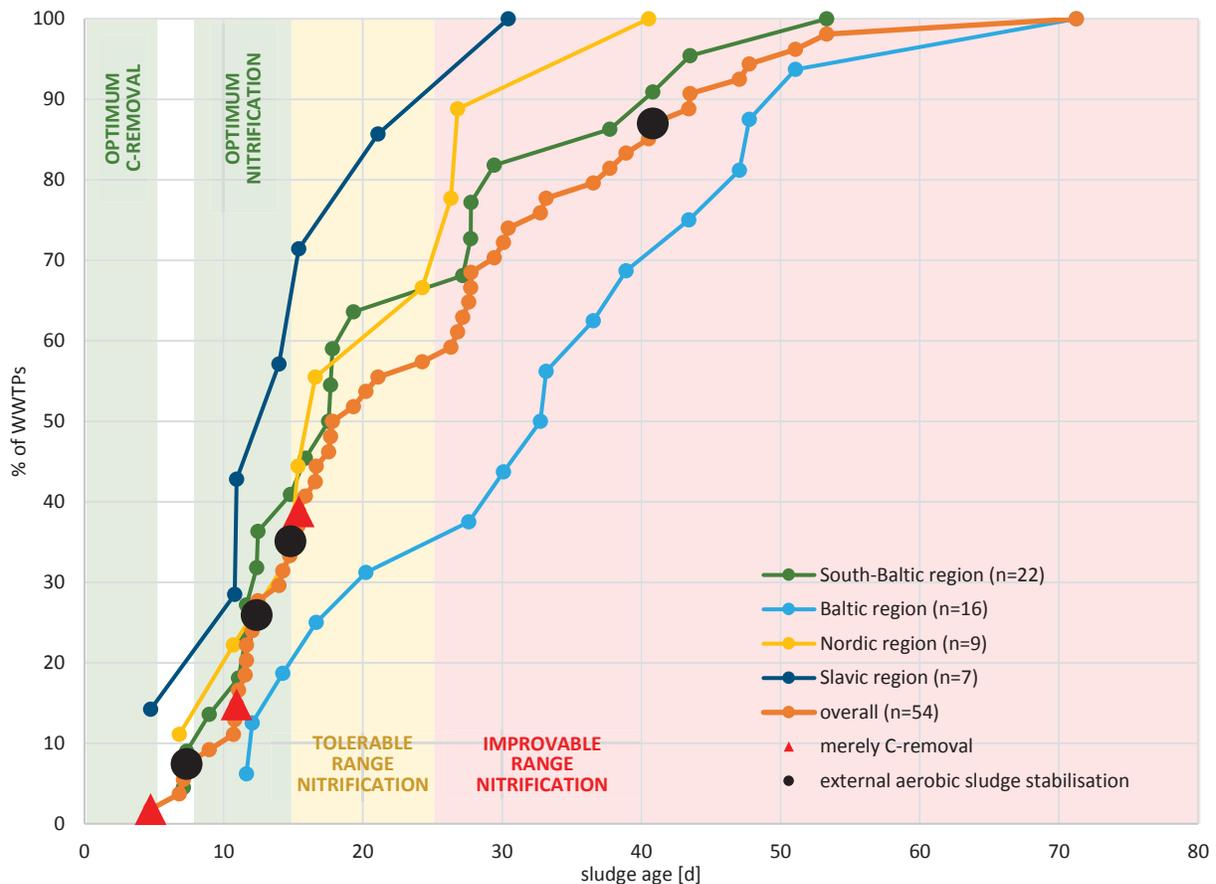
Figure 10 – Sludge age based on BOD<sub>5</sub> as overall and regional display
