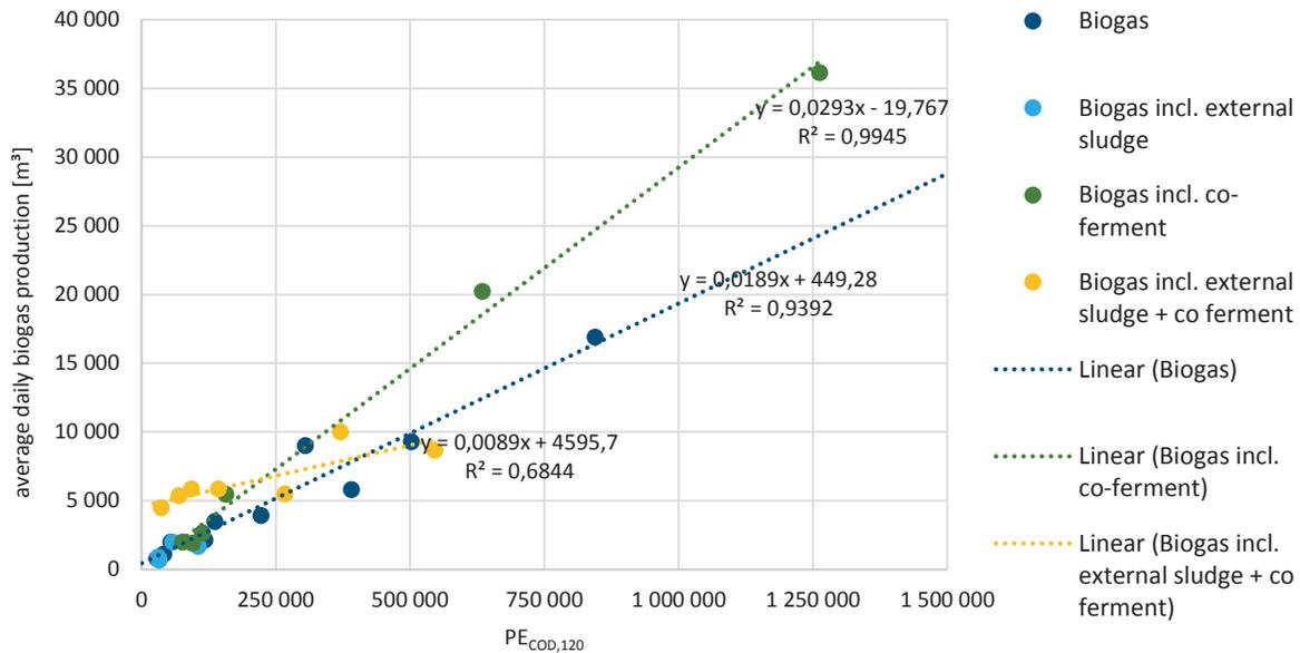
Figure 28 – Average daily biogas production [m³] vs. PE<sub>COD,120</sub>, n=27
