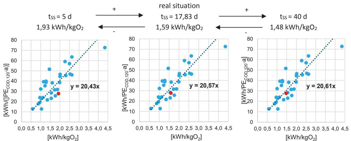
Figure 24 – Impact of sludge age on kWh/kgO<sub>2</sub>
