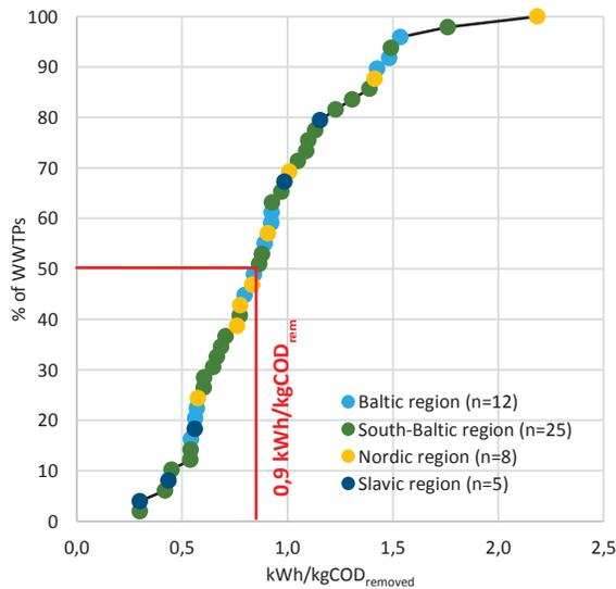
Figure 22 – Specific energy consumption [kWh/kgCOD<sub>rem</sub>], accumulative
