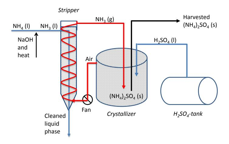
eco:N: stripping + small scale crystallization + crystall harvesting
