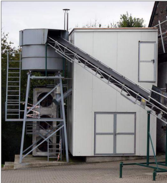
Gasifier for wood + HTC biocoal GRENOL GmbH, Ratingen
